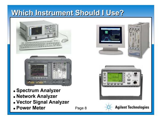
Although a variety of instruments measure power, the most accurate instrument is a power meter and a sensor. The sensor is an RF power-to-voltage transducer. The power meter displays the detected voltage as a value of power in log (dBm) or linear (watts) units. Typical accuracies of a power meter will be in the hundredths of a dB, while other instruments (i.e., spectrum analyzers, network analyzers) will have power measurement accuracies in the tenths of dBs or more.
